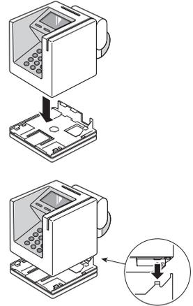
Then carefully push the terminal backwards until the locking mechanism clicks.
