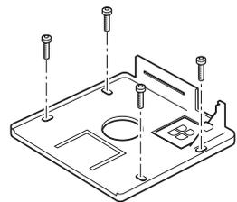
Screwing down the fixing plate
