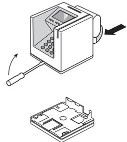
Slightly depress the locking mechanism
